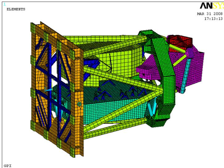
Figure 3: FSS finite element model
