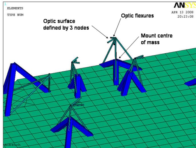
Figure 4: Optical Element Representation in FEM
