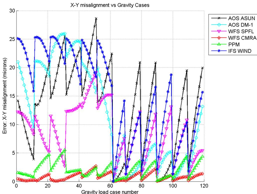
Figure 10: Optical misalignment (X-Y translation of chief-ray) due to gravity flexure
