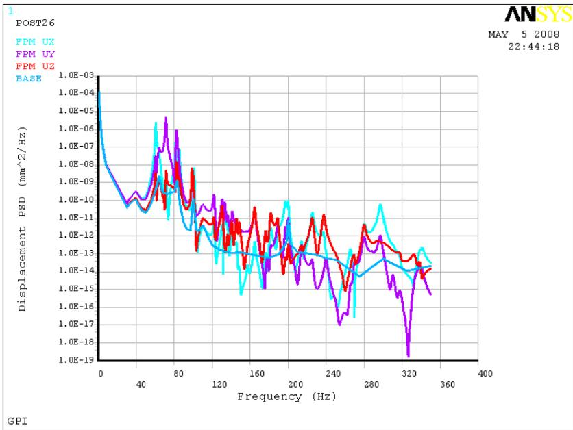
Figure 7: Displacement response PSD at FPM
