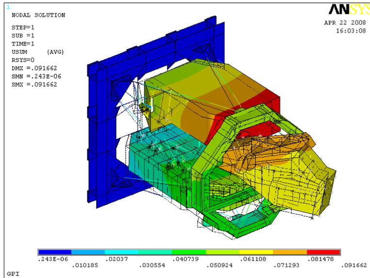
Figure 5: Gravity flexure (X direction)
