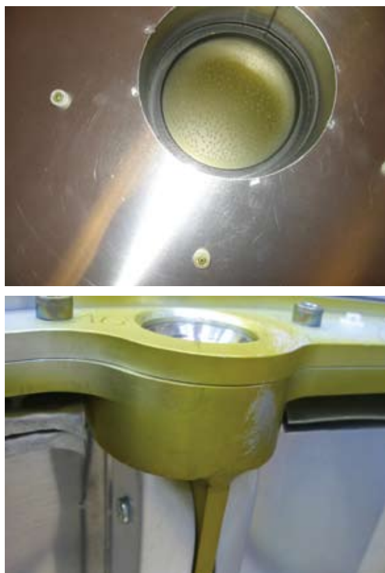
Figure 1. Top image: the contaminated entrance window from inside the dewar. The screw heads and inner baffle also show signs of the discolored contamination seen more clearly in the bottom image of the GNIRS interior. Small areas of the contamination have been cleaned off for illustration.
