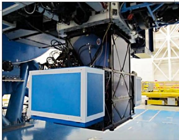
**Figure 22.** Close-up of GPI attached to the instrument support cube (white, at top). Vibrations from the instrument’s cold heads coupled very efficiently into the cube and then into the mirror cell.
