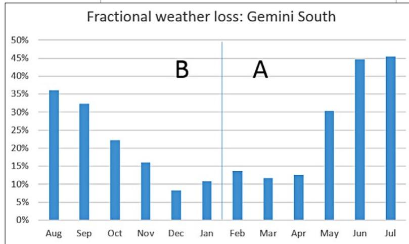
**Figure 19.** Percentage of time lost to weather at Gemini South. This pattern is quite reproducible from year to year. We now take better account of it in the time allocation process; we no longer overload the mid-year months (May-September), and allow more programs into the southern summer time.
