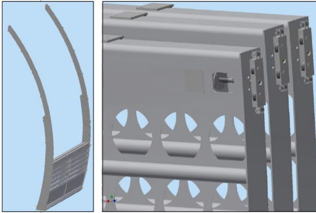
**Figure 15.** The Gemini wind blind design drawings. Left: blind segments all stowed, with the guide tracks above them following the shape of the dome arch. Right: detail of the segments; the largest is 5.5 meters (18 feet) high.
