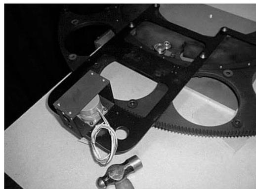
**Figure 17:** Filter Wheel with Motor Mounted
