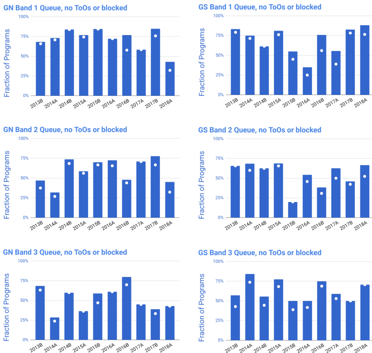
Figure 3.1.1-1: Completion statistics for GN and GS. 2017B and 2018A are represented by the bars at the right of each group. Bars represent the fraction of programs achieving 80% completeness; white dots represent the fraction achieving 100%. Band 1 completion rates in the final two semesters will increase as all Band 1 programs have “persistence”.
