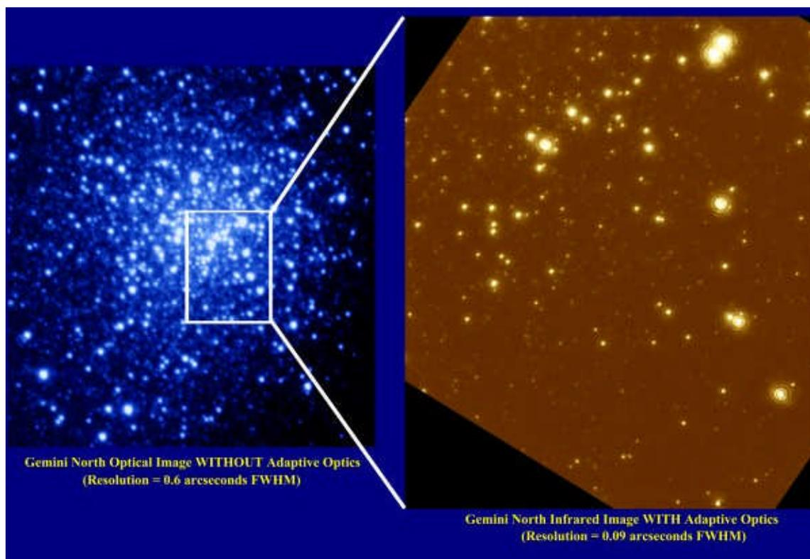
Figure 1: The globular cluster NGC6934 imaged in the visible with the GEMINI acquisition camera (left), and with the Quirc IR camera and the UH-AO system Hokupa'a (right) is one example of the outstanding image quality already obtained at the Gemini telescope.
