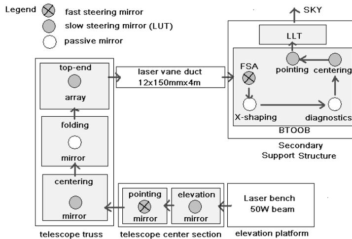
Figure 1: BTO block diagram showing active/passive elements
