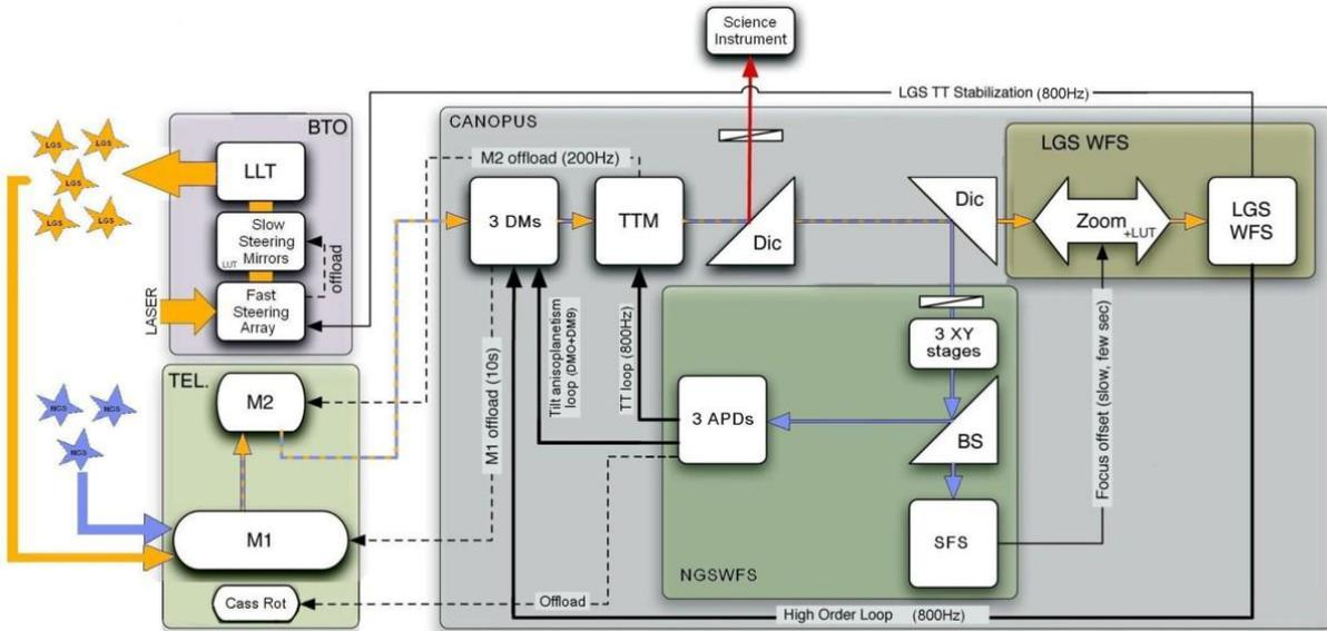
Figure 2: Canopus system block diagram showing control loops
