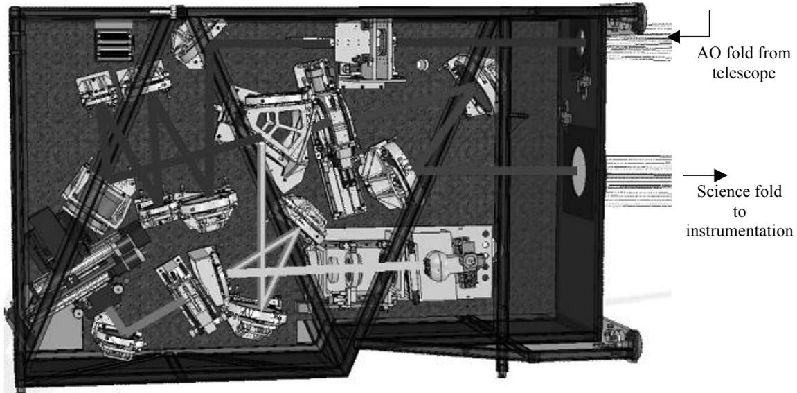
Figure 1. Schematic representation of the three main light paths in Canopus: the input beam from the telescope (blue), the natural guide stars path (red), the laser guide stars path (orange), the corrected output beam for science (light blue).
