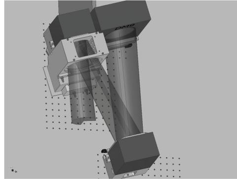
Figure 8. 3D model of the turbulator mounted in front of DM0
