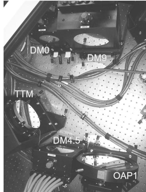
Figure 4. DM9 on interferometer test rig (left) Deformable mirrors mounted on the bench. (right)
