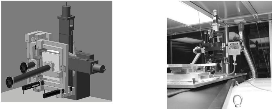
Figure 6. DWFS design study (left) Final assembly installed on Canopus (right). The turbulator hot air exhaust tube and fan – attached to the clean room's roof – can be seen in the background.
