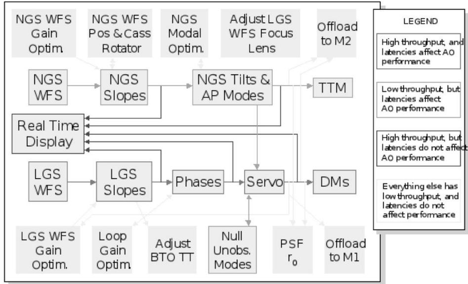
Figure 12. Real Time Controller processing functions (\*)
