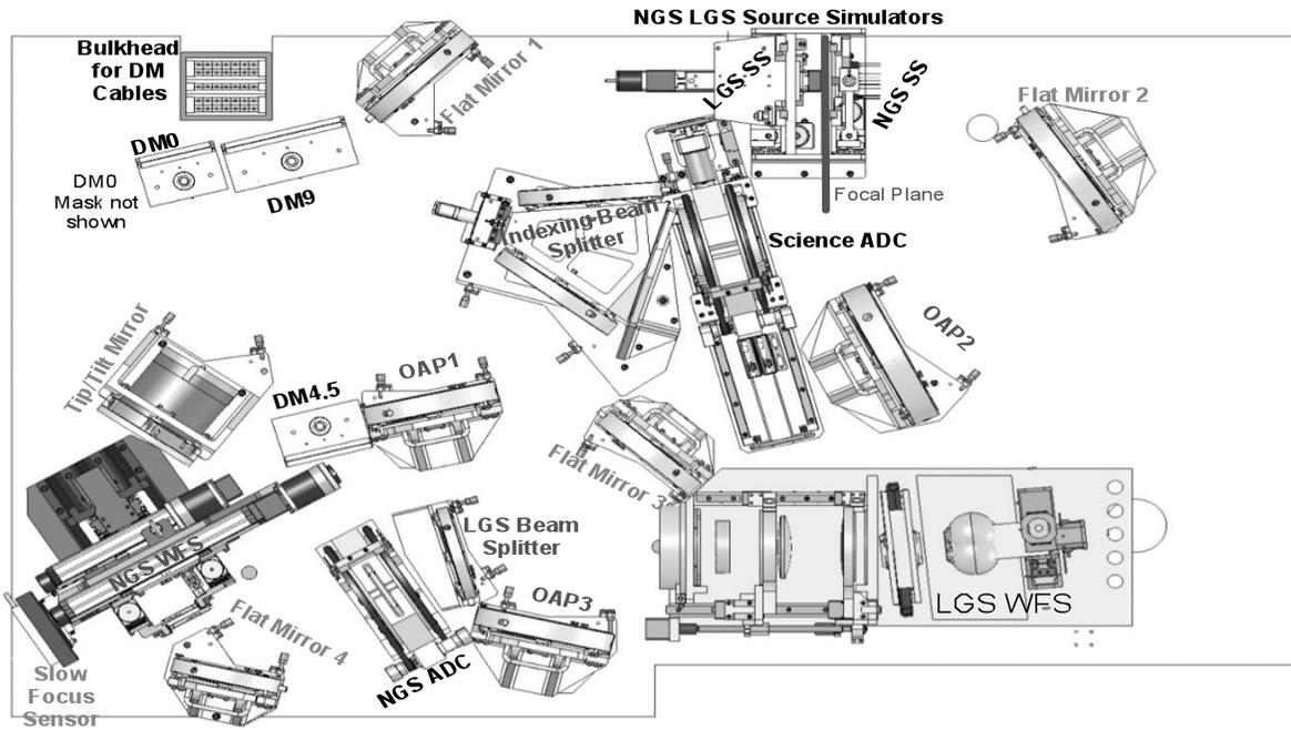
Figure 2. Principal components mounted on the Canopus bench.
