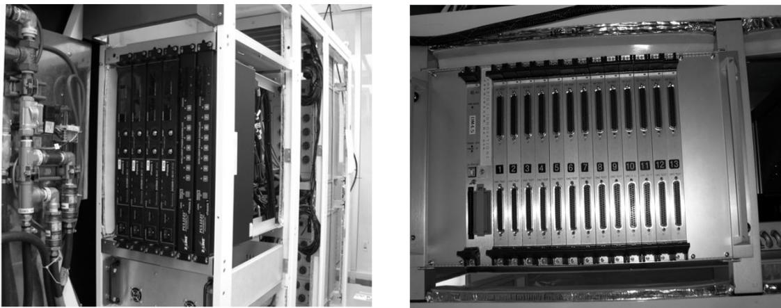
Figure 5. DMs Electronics. HV Power Supplies and Programmable Power Sequencers (left). DM 4.5 HV Driver Boards Rack (right).
