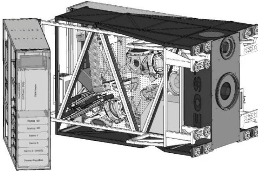
Figure 3. Canopus support structure, +X panel shown opened providing access to the optical bench.
