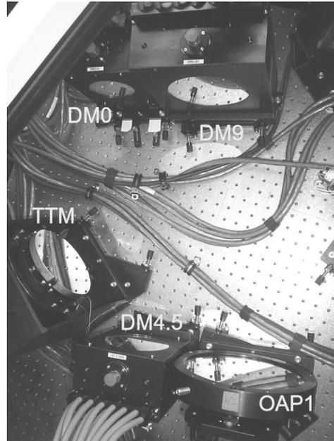
Figure 4. DM9 on interferometer test rig (left) Deformable mirrors mounted on the bench. (right)
