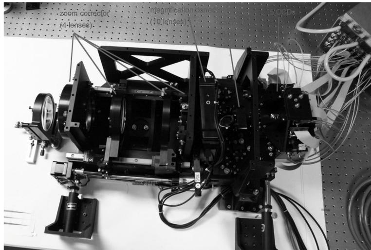
Figure 11. Laser Guide Star Wavefront Sensor Assembly
