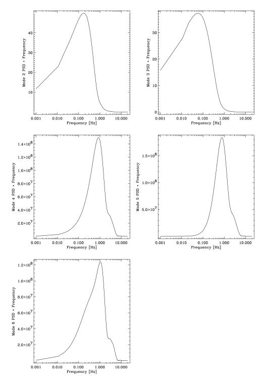
Figure 1: Spectra of the Null mode coefficients  ${\cal A}_2$  through  ${\cal A}_6$
