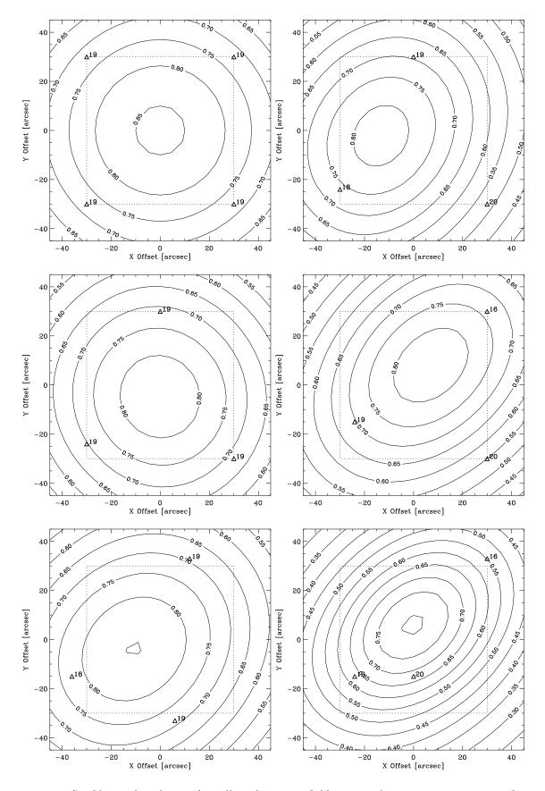
Figure 5: Strehl ratio loss due to the null modes versus field position for various guide star configuration and magnitudes, as plotted on the figures (triangle).
