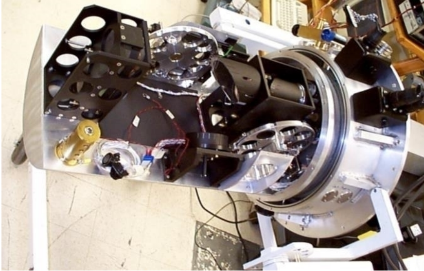
Figure 46: ANDICAM with vacuum shell removed showing optical bench, filter wheels, and dither mirror
