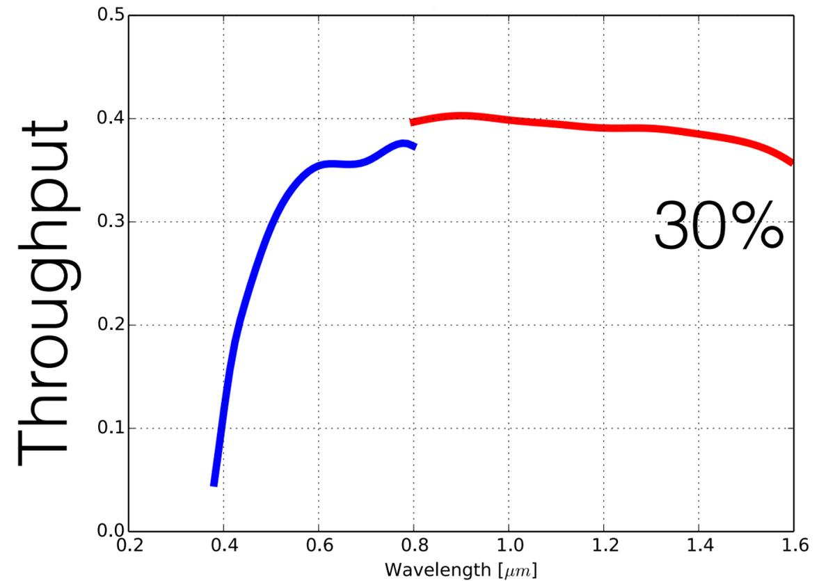
$$M1 \times M2 \times \text{Atm} (1.2) \times 20\% \text{ Slit loss} \times \text{Efficiency}$$
