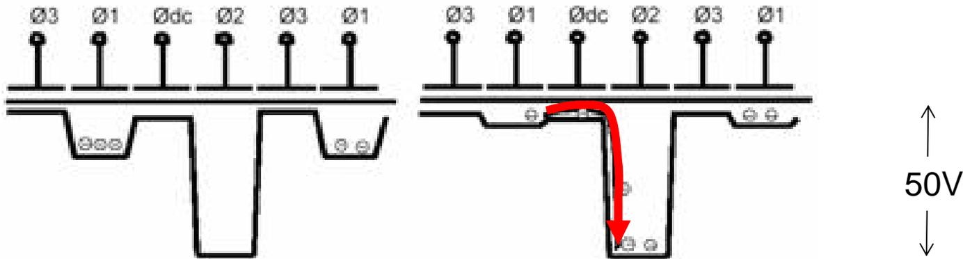
With 40-50V on  $\phi_2$  electrode, conduction band electrons falling into potential well gain enough kinetic energy to sometimes dislodge a valence band electron.
