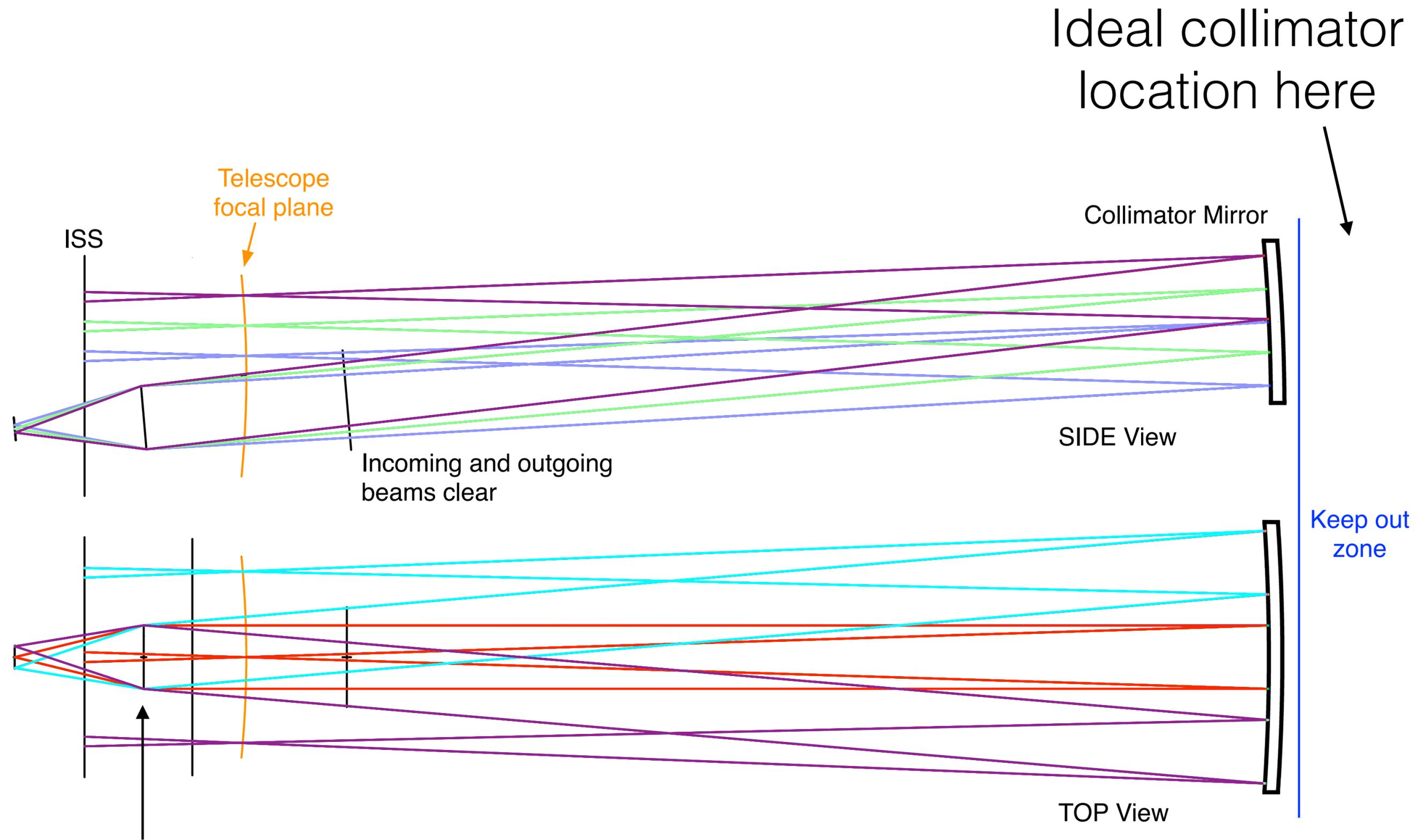
$$\text{Pupil Diameter} = \text{Collimator distance} / (f/\#)_{\text{telescope}}$$
