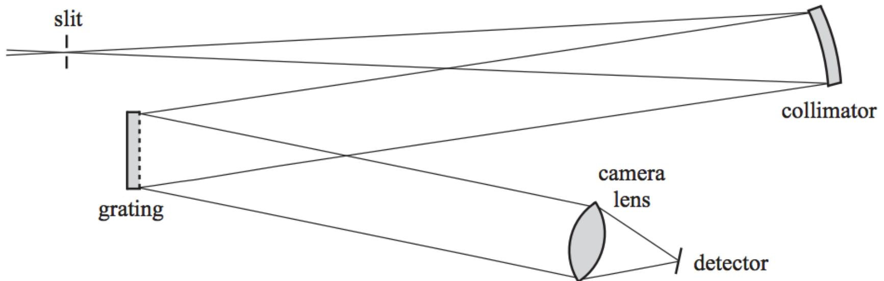
Fig. 1.— The essential components of an astronomical spectrograph.
