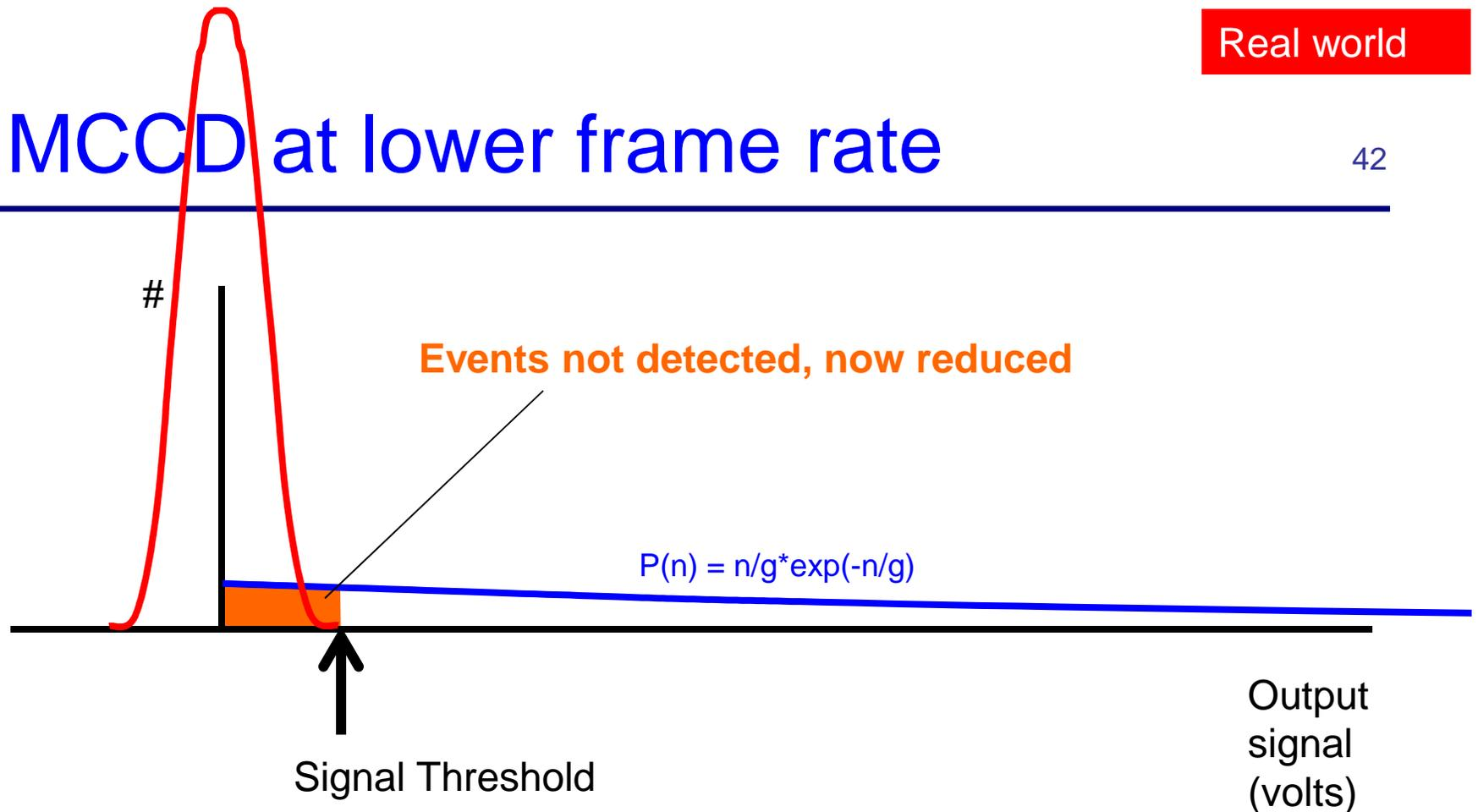
Lower pixel rate → **reduce output noise** to improve counting efficiency.
