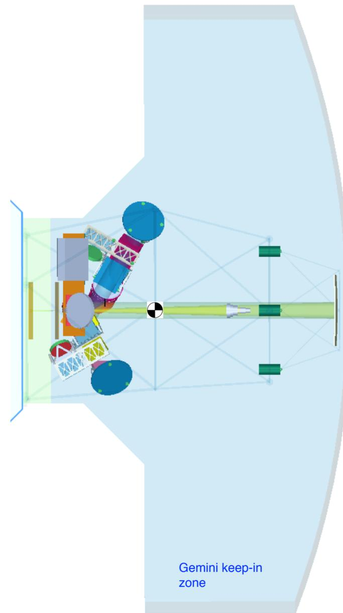
100 mm collimator-to-keep-out-zone distance
