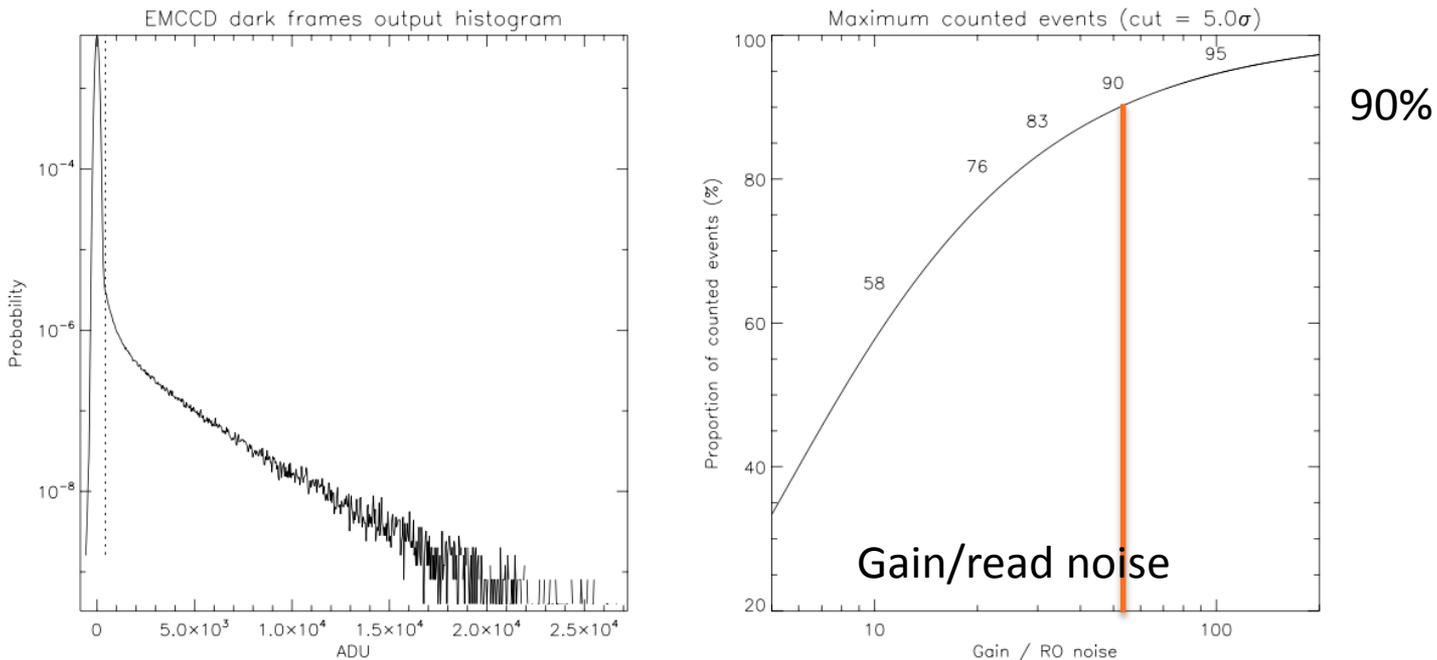
Figure 1. **Left:** Histogram of an EMCCD operated under low flux, at an EM gain of  $\sim 2750$ . Only a few pixels underwent more than one event per frame. The vertical dotted line shows the threshold at  $5.5\sigma$ . The mean event rate is 0.0018 event per pixel per image. **Right:** Proportion of counted events as a function of the ratio of the EM gain over the readout noise. A cut level of  $5\sigma$  is used. Values for ratios of 10, 20, 30, 50 and 100 are printed.
