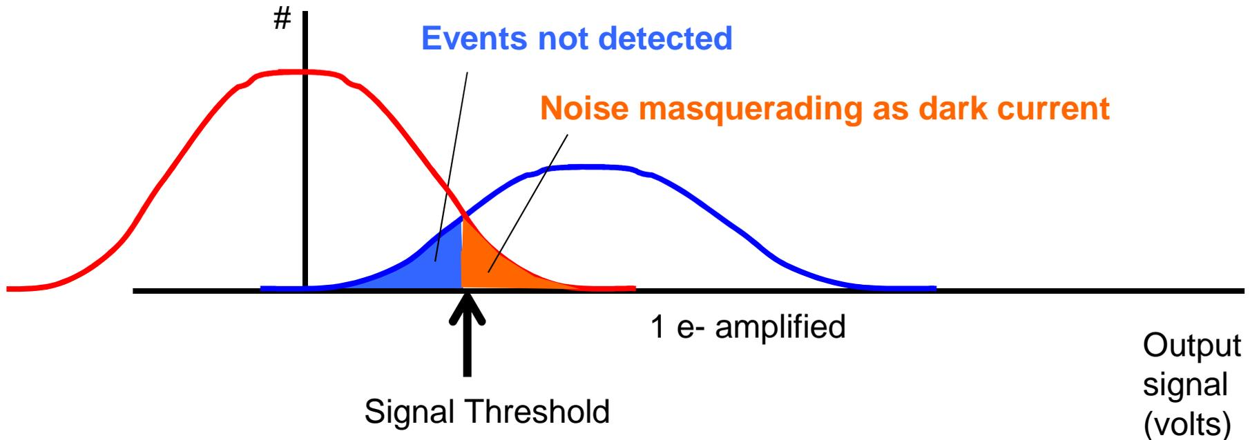
Attempting to recover these real events by lowering threshold results in elevated dark counts due to electronic noise.
