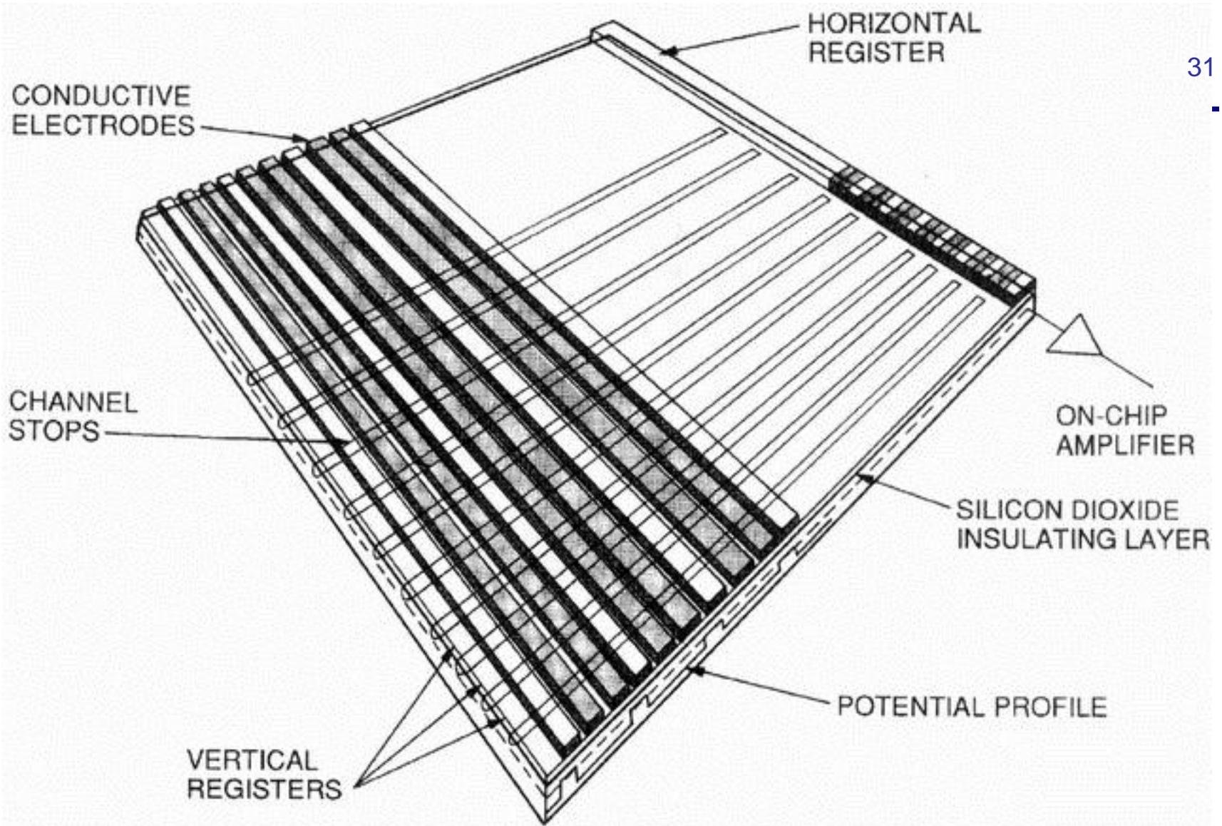
Primary components that make up a three-phase CCD.
