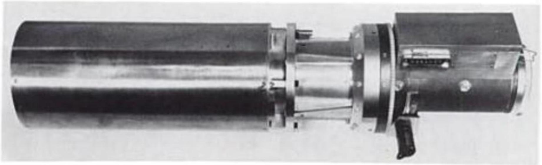
**Fig. 19.5. The IPCS detector head unit, containing image intensifier, coupling lens and television camera.**
