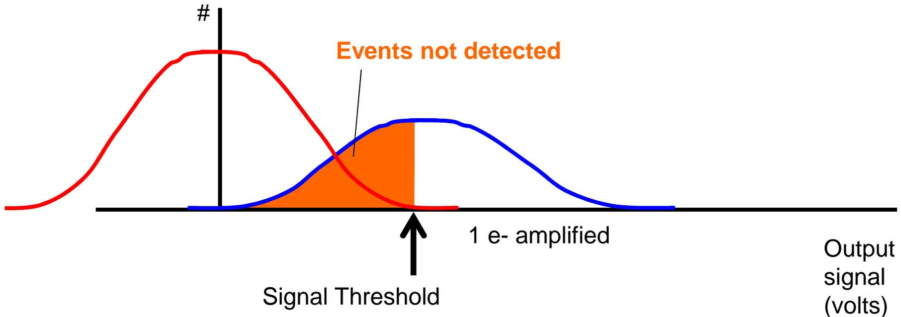
The higher frame needed to avoid coincidence losses requires higher bandwidth output amplifier (faster settling)
