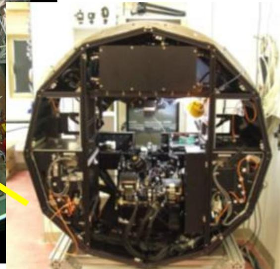
The Pyramid wavefront sensor in the AGW unit
