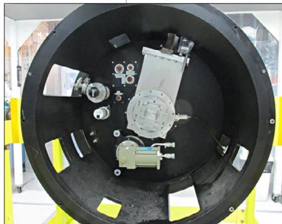
all mechanisms, which raised some additional suspicions during the movement of the Multi-Object Spectroscopy (MOS) wheel (Figure 14). Further inspection indicated significant wear in some of the ball bearings, so all were replaced. The team then reassembled and successfully tested the entire mechanism.
