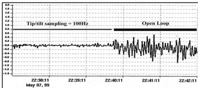
**Figure 2:** Tilt loop performance graph
