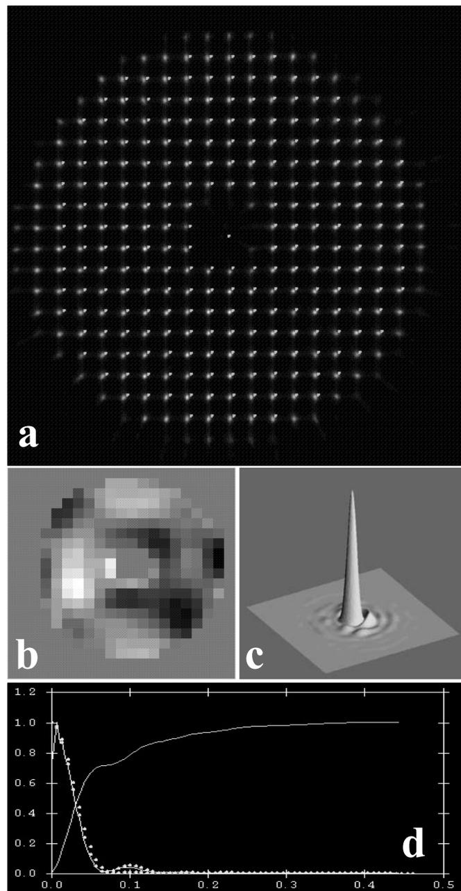
**Figure1 (a-d):** Prime focus wavefront sensor image (a) and data reduction (b-d). Image (a) shows the Shack-Hartman spot pattern of a star with (smaller) reference spots, (b) is an optical path difference map, (c) shows a 3-D point spread function (psf), and (d) is a plot of encircled energy vs. diameter in arcseconds.
