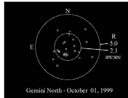
**Figure 3:** Pointing results revealing better than 3 arcseconds rms.
