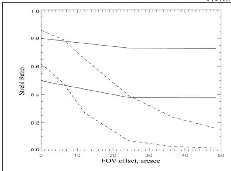
**Figure 2:** J (lower curves) and K (upper curves) Strehl ratio versus off-axis angle for Natural Guide Star systems (dashed line) and for a MCAO system using 5 LGSs, 4 NGSs and 3 deformable mirrors (solid line). Both are 12x12 subapertures Shack-Hartmann systems. This case was run for a zero degree zenith angle, under median seeing conditions, for a typical Cerro Pachón turbulence profile.
