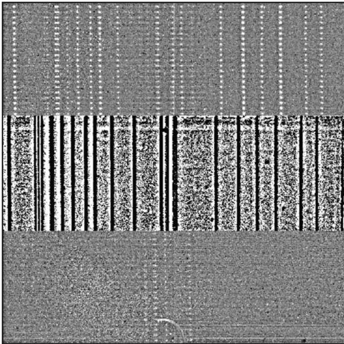
*This mosaic of 3 COHSI exposures shows: Top - the spectra of the Mauna Kea night sky with the grating offset so that the OH lines are not blocked at the mask. Middle - the mask illuminated directly (not through the fibres). The AR coated mask features are clearly seen. Bottom - the suppressed night sky. Some weak oxygen lines which have no mask features are clearly seen.*
