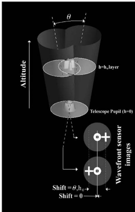
**Figure 1:** Principle of MCAO. The shift of a phase feature signature in the 2-D wave-front sensors is proportional to the altitude of the atmospheric layer which created it. Once reconstructed, the 3-dimensional phase volume is then compensated in a 3-D fashion by using several deformable mirrors conjugated at a range of altitude.
