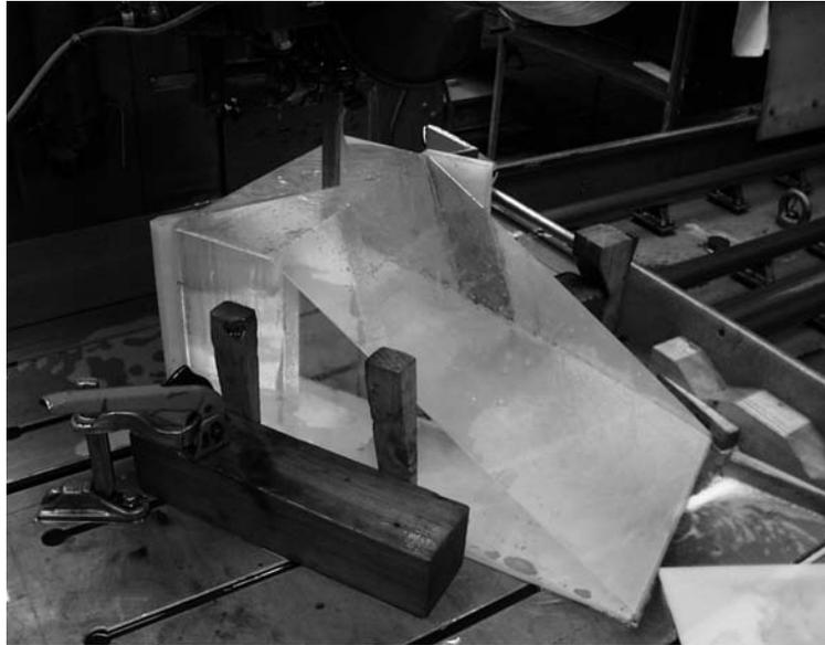
**Figure 1:** Cutting of the large fused silica prism ("immersion prism") at Heraeus. The prism was cut out of a single large rectangular block 612x375x370mm in size and is made out of the highest homogeneity fused silica commercially available (less than 1 part per million variation in the refractive index).
