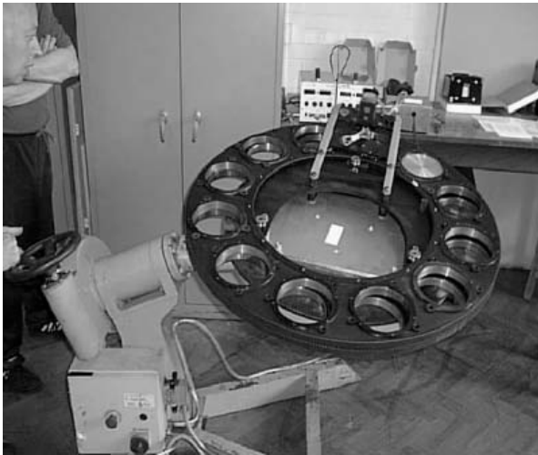
Figure 9 - Filter wheels undergoing flexure testing at Durham
