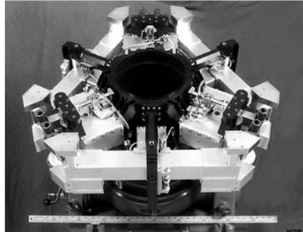
**Figure 7.** Secondary mirror tilt mechanism at Lockheed, August 1997.
