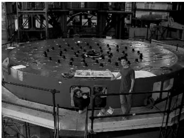
Figure 6. The first M1 cell during installation of the mirror support system, August 1997.
