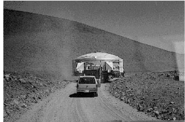
Figure 3. Transportation of the Mauna Kea Coating Plant up Mauna Kea, August 1997.
