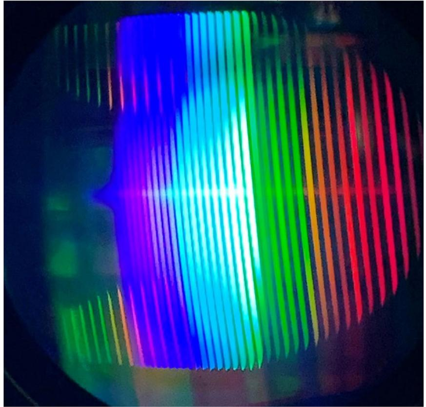
The spectrograph subsystem is a gravity-stable asymmetric white-pupil échelle spectrograph, with two arms and volume-phase holographic grating cross-dispersers. It comprises the following key elements:
