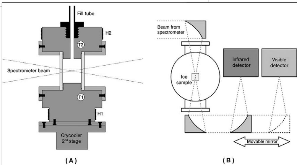
Figure 2 represent the spectrometer beam through the sample. Thermometers (T1 and T2) and heating elements (H1 and H2) control the temperature of the sample down to 30 Kelvin (K). Further details concerning the cell are described in Tegler *et al.* (2019).
