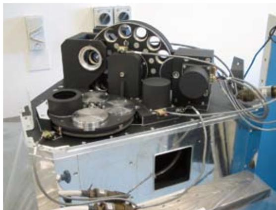
**Figure 1.** The cold structure of GSAOI is shown. The large vertical wheels house the instrument’s filters, while the horizontal wheel is intended to hold focal plane masks. The bench and passive radiation shields on its perimeter are all derived from the design of NIRI.
