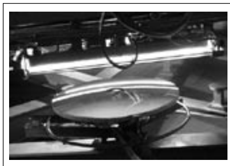
Figure 1: The Gemini South secondary mirror passing under a magnetron, which applied the reflective silver layer in the vacuum coating chamber during the silver coating process on October 9, 2003. Gemini Observatory photo by Gustavo Arriagada
