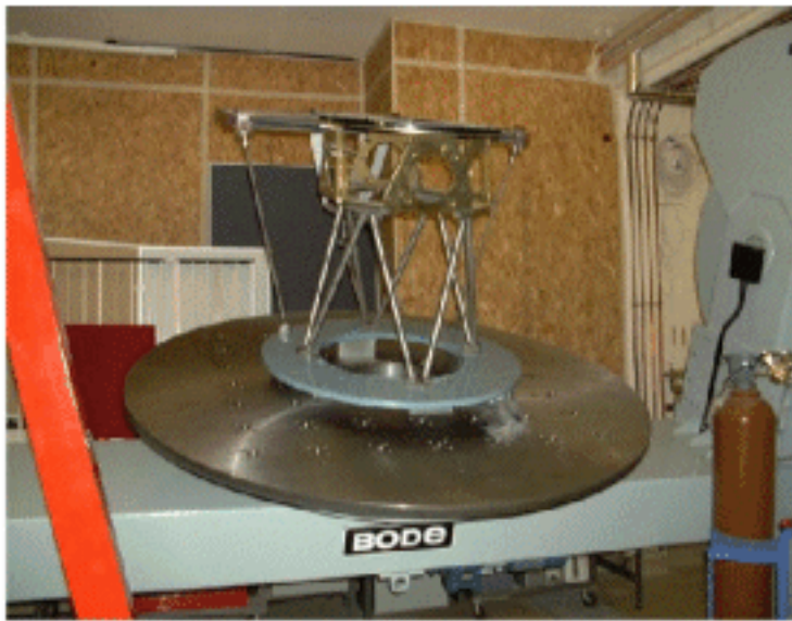
Figure 15. Telescope Simulator modified to accept GMOS and Michelle.
