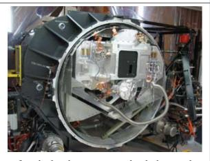
surfaces that have been contaminated with plastic residue. Some optics may be recoated or repolished, if necessary, after the cleaning process is complete. We will also look for ways to make improvements to GNIRS while it is being overhauled, taking advantage of this unique opportunity to examine every part of the instrument without impacting the observing schedule.
