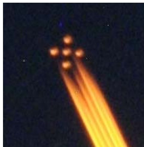
Figure 4.5 - The recent "first light" for the Gemini-S laser launch system is captured by this photo (made by Maxime Boccas, Gemini). Projecting a constellation of laser beacons into the sodium layer was a first in astronomy and will help enable incredible research opportunities for Gemini's science community.
