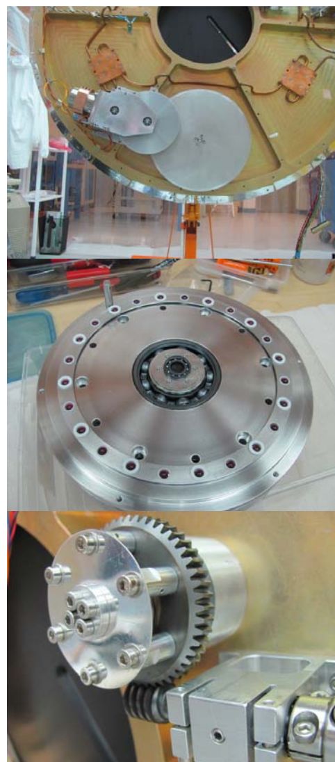
Figure 4.9 – (Top) The new MOS drive assembly, which was designed, built, and installed by Gemini engineering, is seen in the above photo. (Middle) The new MOS wheel hub, featuring new tapered roller bearings for smoother operation and concentric rings of ruby bearings for improved thermal conductivity across the hub is seen. (Bottom) The new Decker worm gear drive assembly is shown.
