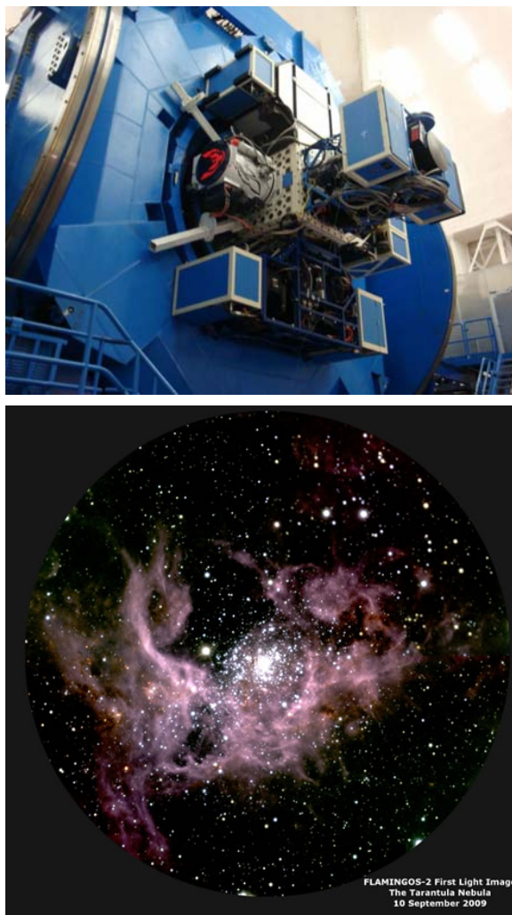
Figure C.12 – FLAMINGOS-2 was delivered in 2009 to Gemini-S, where it is currently being commissioned, in anticipation of being released for community use in 2010. Shown above is FLAMINGOS-2 on the up-looking port of Gemini-S. Shown below is one of the first light images recorded with FLAMINGOS-2 of the Tarantula Nebula.
