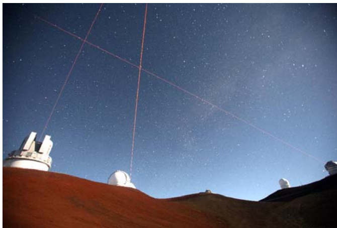
Figure D.7 – Laser AO operations on Mauna Kea are arguably the most advanced on any site worldwide, as demonstrated here with sodium lasers being concurrently propagated by Keck, Subaru, and Gemini. The considerable experience Gemini is gaining from the ALTAIR LGS system is being incorporated into MCAO at Gemini-S. Photo credit: Subaru Observatory
