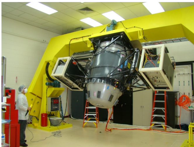
Figure C.13 – GNIRS is shown on the HBF flexure rig, undergoing an extensive series of tests before it is deployed on Gemini-N in 2010.
