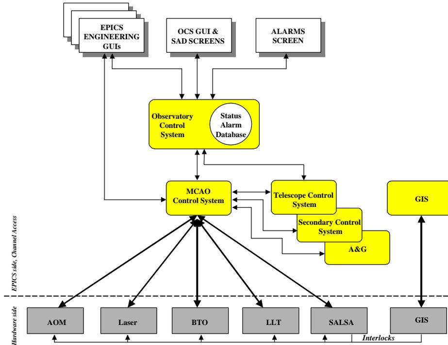
Figure 4: Relative position of the MCAO CS in the Gemini Observatory
