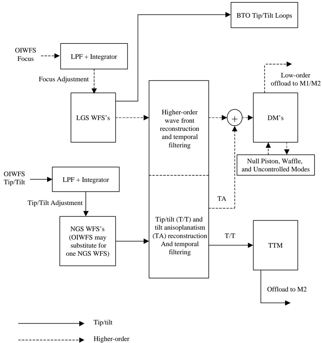
Figure 3: MCAO Control Function Schematic.
